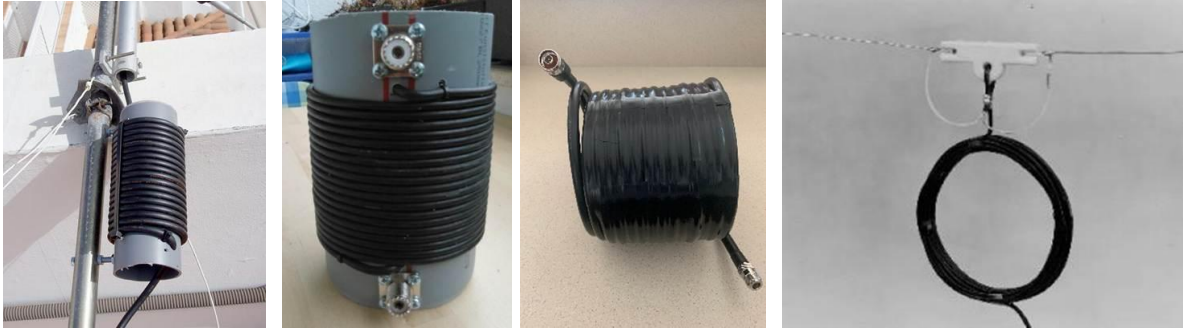
Figure 3a. Figure 3b. Figure 3c. Figure 3d. Air-wound Coaxial Cable Choke or Big Ugly Balun. BUILD AN AIR WOUND 1:1 CHOKE BALUN FOR HF – THE UGLY BALUN!
