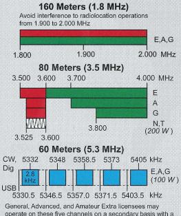
operate on these five channels on a secondary basis with a maximum effective radiated power (ERP) of 100 W PEP relative to a half-wave dipole. Permitted operating modes include upper sideband voice (USB), CW, RTTY, PSK31 and other digital modes such as PACTOR III. Only one signal at a time is permitted on any channel.
