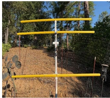
Test Setup w/CM Chokes using a calibrated 15' piece of RG-316
