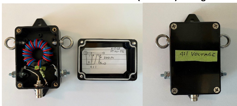
Finished 4:1 Ruthroff Voltage Balun Transformer Wound on a FT140-43 Core
