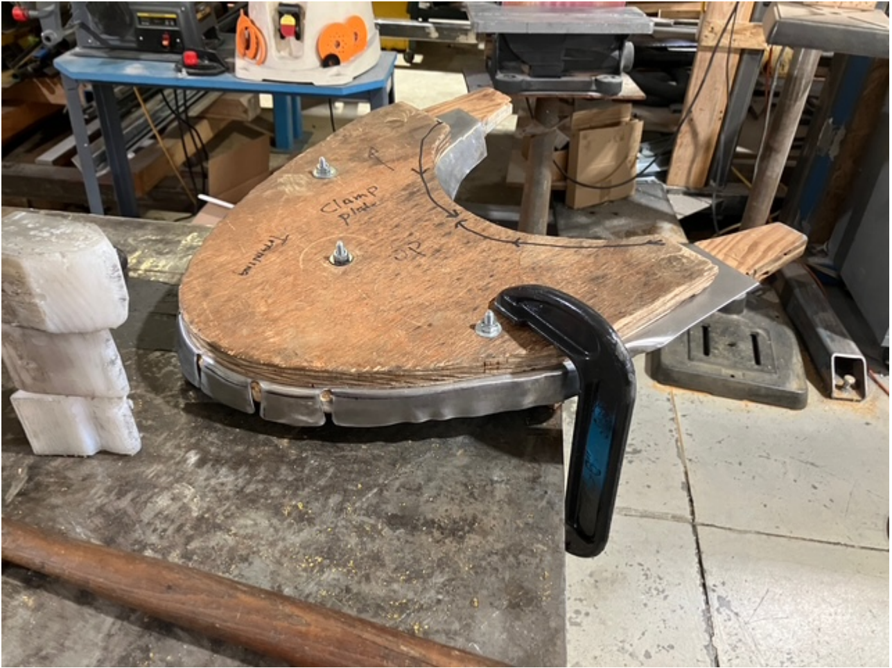
A wooden mold set for metal fabrication on the wing
