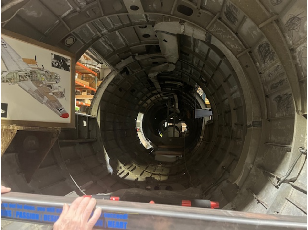
Tail section ready for restoration process
